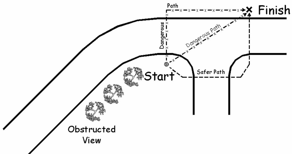
**Complex intersections** - Cars at more complex intersections approach from three or more directions. It is usually difficult to see every potential vehicle approach from any one location. Offset intersections provide an even more complicated set-up.
